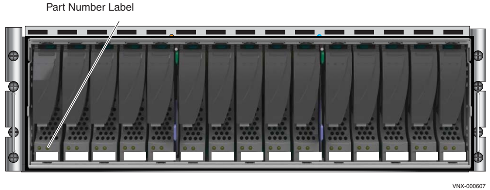
Figure 34 Example of the 3U, 15 (3.5-inch) disk drive DAE (front view)
